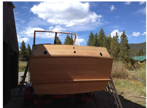
A big step—new transom installed!
